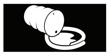
Contain the spill area with sorbent socks, to prevent expansion or additional contamination.
